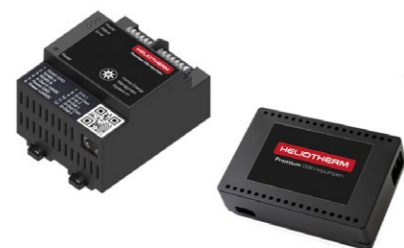
HEMS-Gateway enables direct and secure communication with on-site devices
